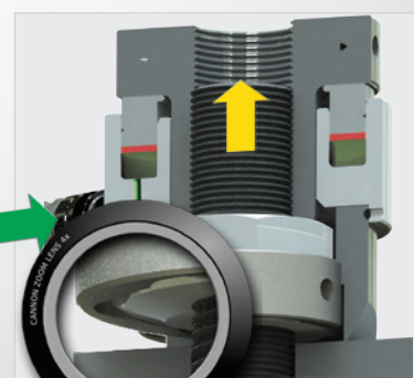
The tensioner is pressurised to the pre-calculated value. Bolt load is directly proportional to hydraulic pressure. The bolt stretches and a gap is formed below the hexagon nut. Once the target pressure is reached, the pressure is held.
