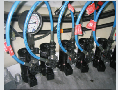
360° degree swivel action ensures that the hoses are positioned where you want them.
