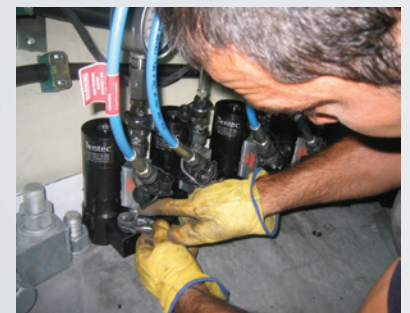
Geared Nut Run-Down, allows for rapid seating of hexagon nut.
